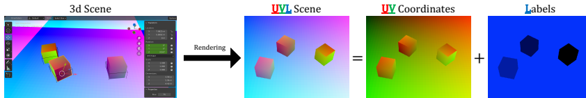
Figure 3: A scene is obtained by rendering a 3D state into an image, where the first two color channels represent u, v coordinates and the third channel l represents object labels.
